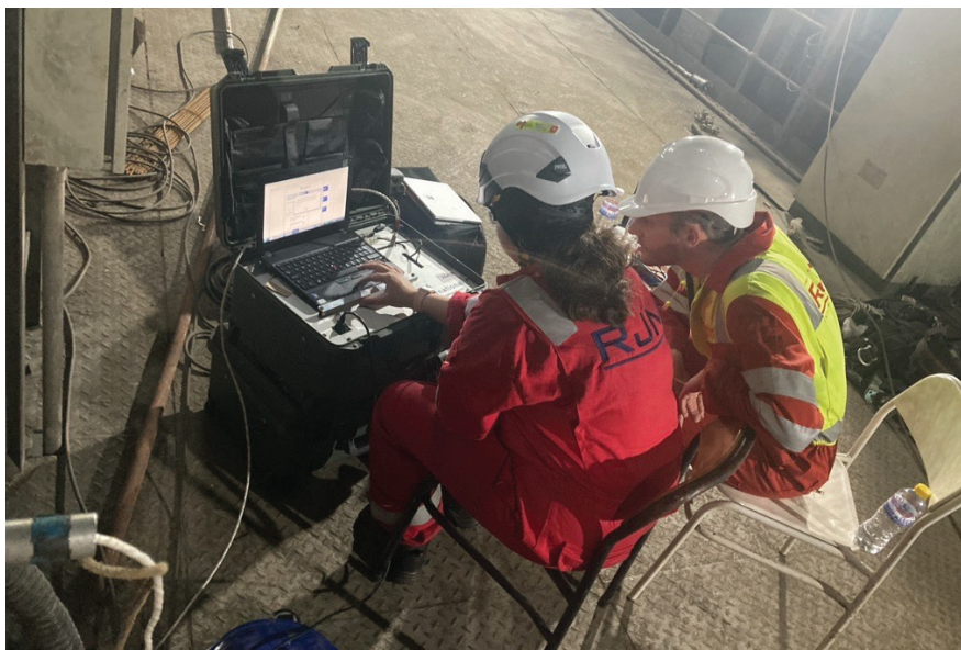
Measuring air flow distribution as part of the preliminary project work
